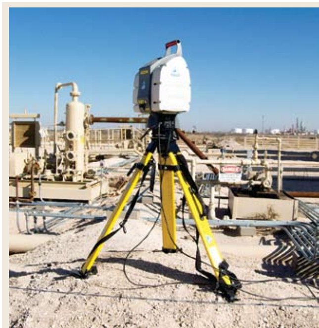
Fig. 1. A laser scanner can capture images above and below, close up or from 300 yards away.
